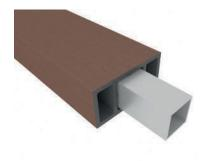
Pre-drill galvanized square pipe and WPC batten tube at the same time, distance of pre-drill hole should be same distance as pre-drilled hole on wall.
