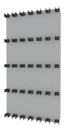
Insert galvanized square pipe into WPC batten tube, galvanized square pipe should be same length as WPC batten tube.
