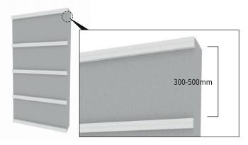
2 Pre-drill metal joist horizontally according to needed distance.
