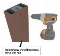
Put batten tube into the U shape fastener, and then use core screw to fix batten tube to the U shape fastener.
