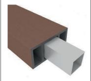
Pre-drill galvanized square pipe and WPC batten tube at the same time, distance of predrill hole should be same distance as metal joist.
